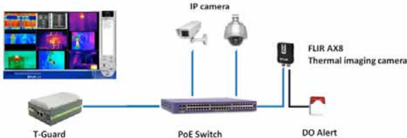
T-Guard makes use of FLIR's AX-8 camera and ADE's AD-TG200 network video recorder. It allows managing temperature-driven alarms triggered by the FLIR AX8 sensor, in addition to other sensor information like IP cameras, voltage measurement and environment temperature measurement.
