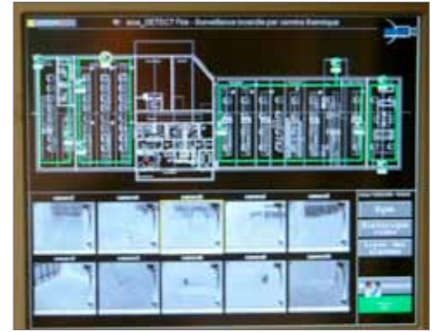
The touch screen interface shows the floor plan of the facility and live thermal video footage of all ten FLIR A310 thermal imaging cameras, including automatic alarms and accurate temperature readings.
