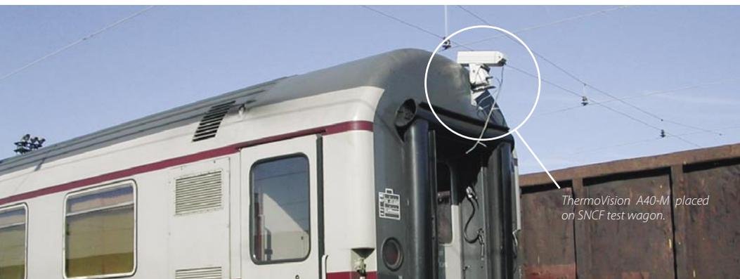
ThermoVision A40-M placed on SNCF test wagon.
