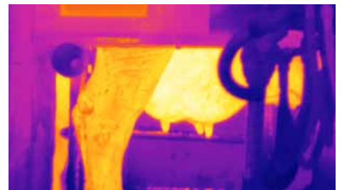
The two FLIR A310 thermal imaging cameras record images of the cow's udder from both sides.
