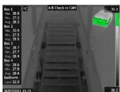
Suitcases do not trigger the alarm, even if the treshold temperature is reached. The percentage of the ROI that reaches that temperature is too small.
