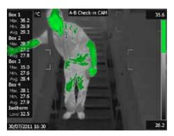
This test shows that if a certain percentage of an ROI reaches the threshold temperature, for instance due to the wave of an arm, the alarm goes off.
