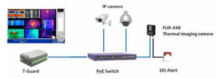
T-Guard makes use of FLIR's AX-8 camera and ADE's AD-TG200 network video recorder. It allows managing temperature-driven alarms triggered by the FLIR AX8 sensor, in addition to other sensor information like IP cameras, voltage measurement and environment temperature measurement.
