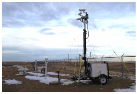
An IntelliView trailer in the field: The weatherproof and self-contained trailer can accommodate multiple DCAM™ units and green power options (fuel cell and solar panels). The DCAM offers an effective way of detecting and alerting on small above-ground fluid spills, sprays and pooling within seconds.
