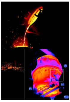
Thermal imaging cameras can detect hot spots on the ladle that warn of a failure far sooner than a visual inspection. This allows the ladle to be taken out of service before failure occurs.
