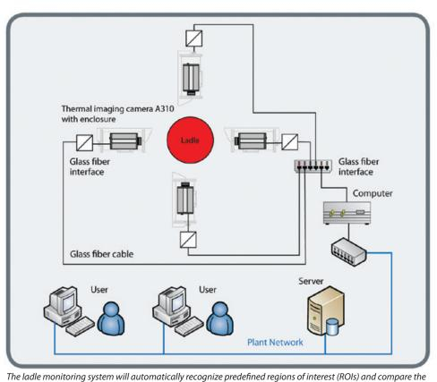
measured temperature with previously set parameters.
