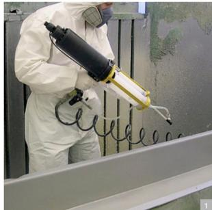
Elastomeric surface treatment for lining longitudinal feeders. Parts protection, noise reduction, feeding optimization and general equipment lifetime extension. FDA approval for use in the pharmaceutical & food sector.
