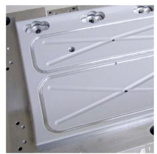
Sprayable elastomeric coatings for the surface protection during plastic welding processes. Precise, true-to-contour, soft and haptic - but nevertheless wear-resistant.
