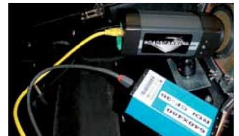
The Road Doctor diagnostics top box contains both a FLIR A-Series thermal imaging camera and a digital video camera.
